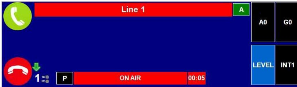
Each line is managed from this window. At the left you can find the buttons to unhook the operator's phone and the line, next to the incoming / outgoing call indicators and displays showing the line number and line send/receive levels.
