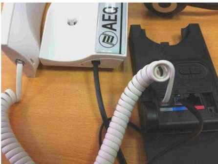
In order to connect one of those headsets, disconnect the micro-telephone 4-pin RJ9 connector from the SYSTEL IP HS body, and connect a RJ9 connection cable to the headset or its base.
