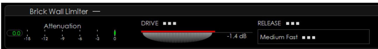
The final stage of the processing is the Brick Wall Limiter. It takes place right before the output, and is the only stage in the chain that cannot be entirely bypassed. Although the Drive can be switched ON and OFF (set to zero) the Brick Wall Limiter will not allow the output of the chain to exceed 0 dBFS.
