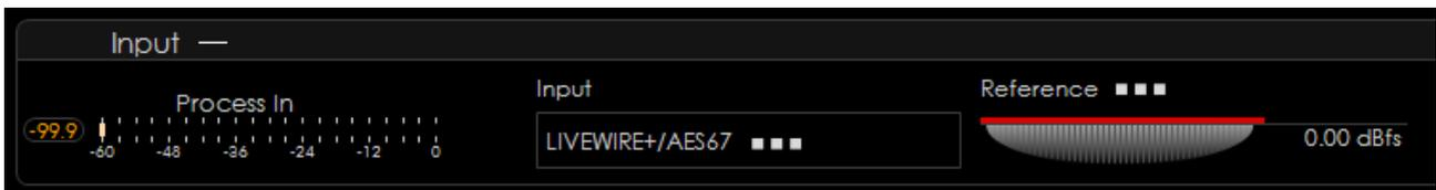
**Process In** – Displays the input level of the processing chain of the currently selected input.
