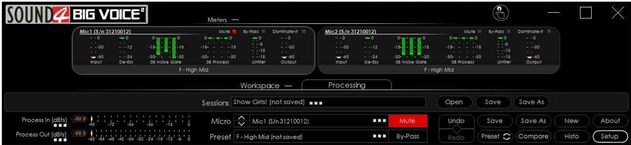
Double click on the desired preset will load it automatically to the device.
