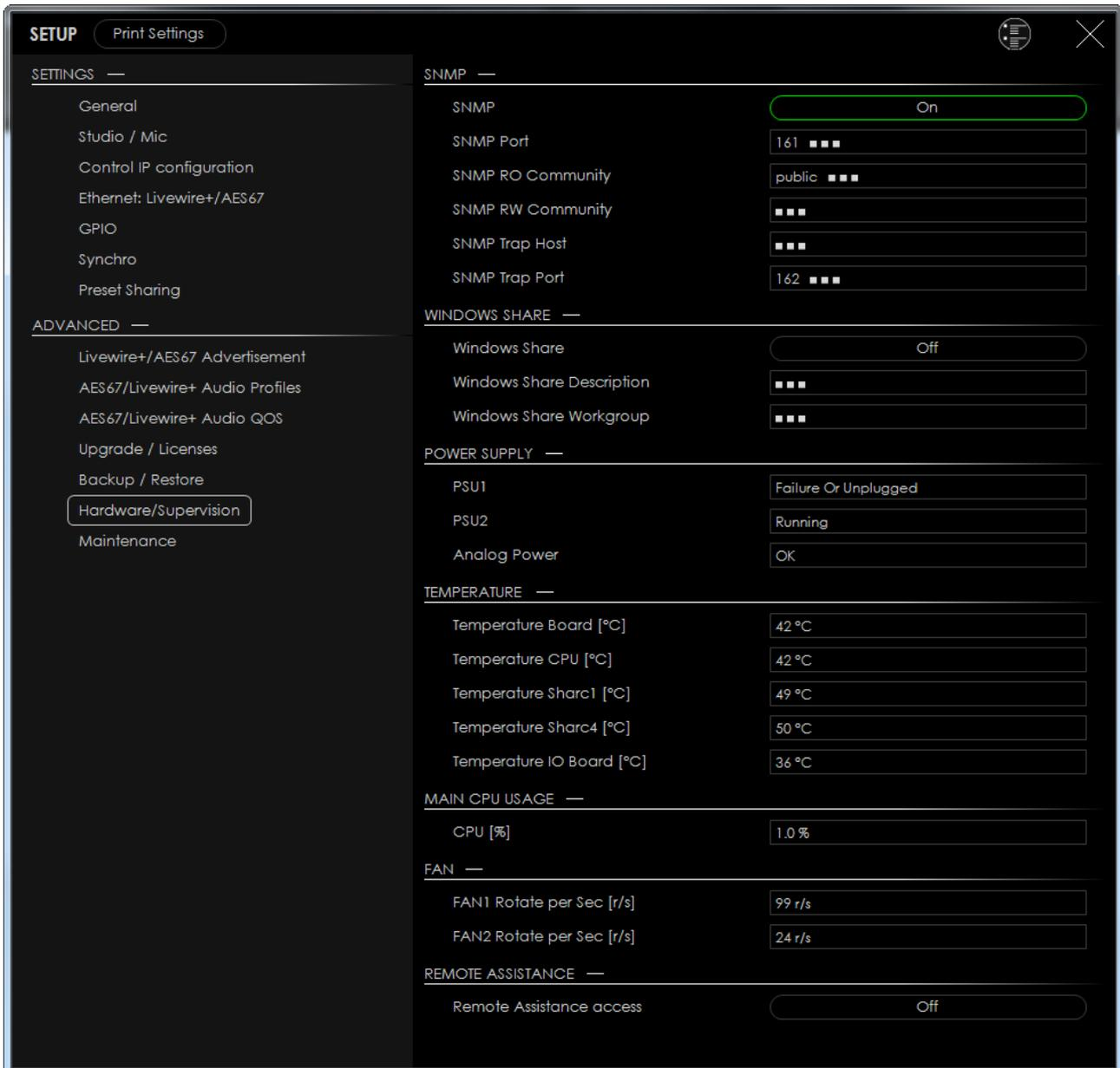
**SNMP** – turn the option [On] or [Off] and specify SNMP Port, SNMO RO Community, SNMO RW Community, SNMP Trap Host and SNMP Trap Port.
