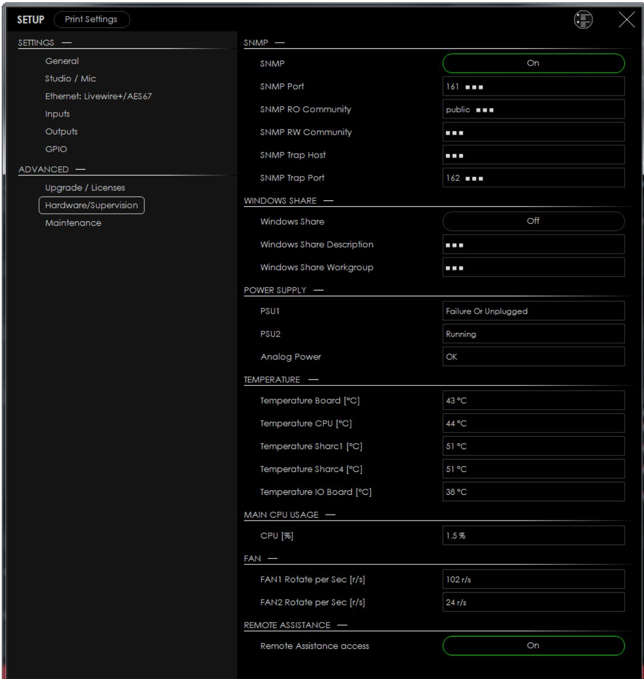
**SNMP** – turn the option [ON] or [Off] and specify SNMP Port, SNMO RO Community, SNMO RW Community, SNMP Trap Host and SNMP Trap Port.
