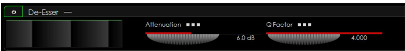
The De-Esser automatically tracks and attenuates sibilants in the audio. The frequency is determined instantly and does not require manual adjustment.
