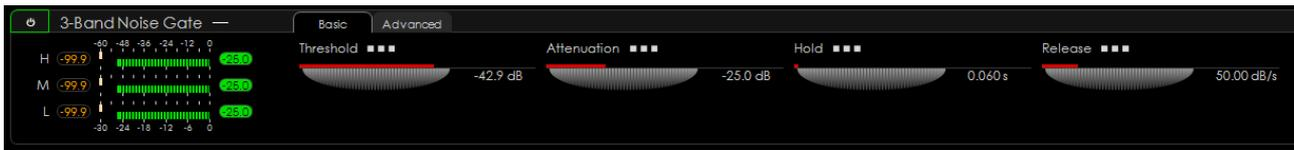
The SOUND4 BIG VOICE<sup>2</sup> - Base has a 3-band noise gate. This can help gate noises in specific bands (for example, noises generated by doors, countertops and etc.) while still passing actual speech. Bear in mind that the attack time on the SOUND4 BIG VOICE<sup>2</sup> - Base gate is virtually instantaneous (set) and is not adjustable.
